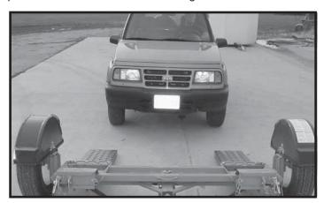
**Step 4.** Before loading (and unloading) towed vehicle make sure platform and towed vehicle are in straight alignment. Tow dolly must be completely and properly hooked up to the towing vehicle. **Towing vehicle must be larger and at least 1000 lbs. heavier than the tow dolly and towed vehicle combined.**
